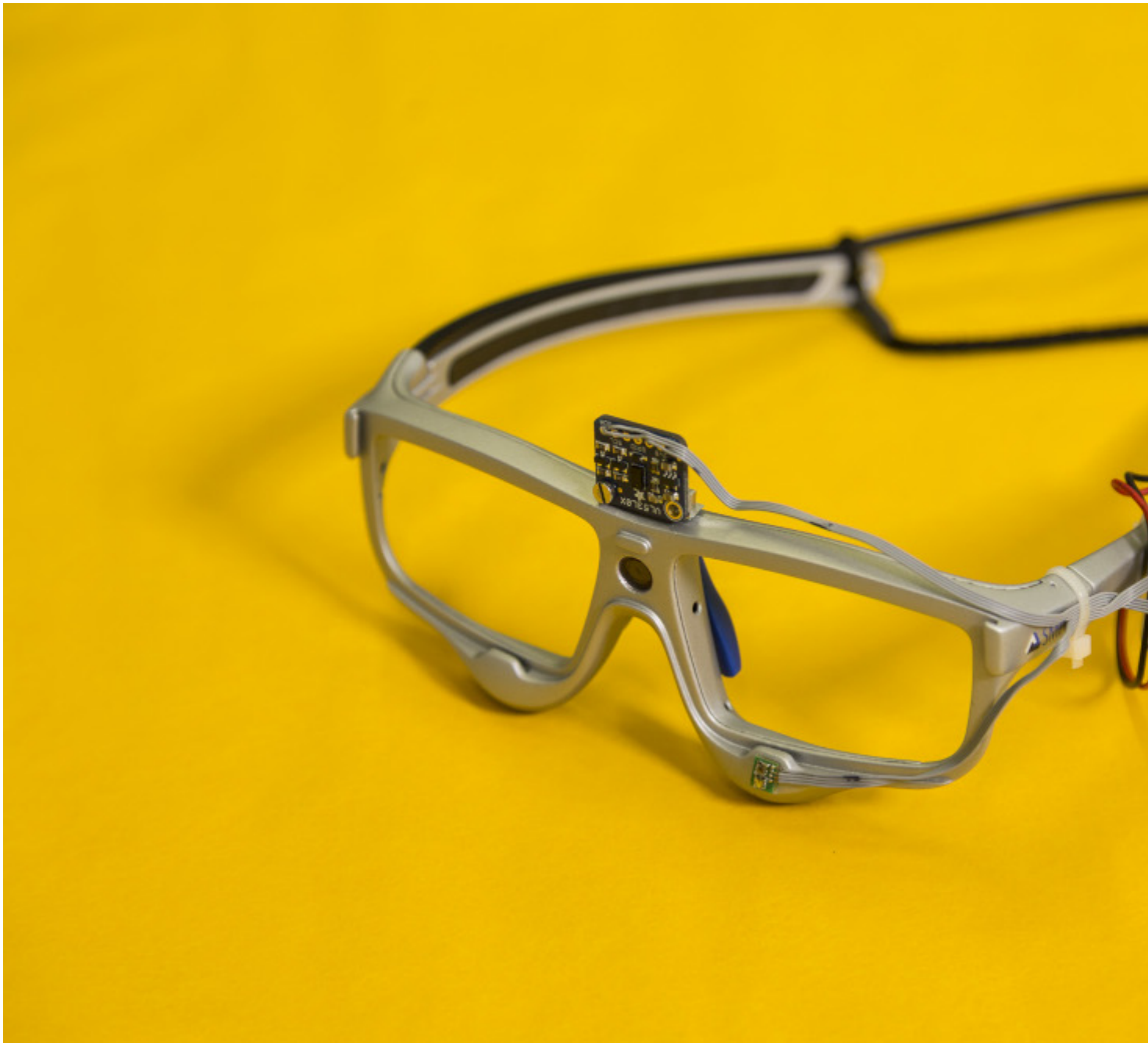
Smart glasses developed by Leung and Schmied, which measure both light effects and eye movements.
