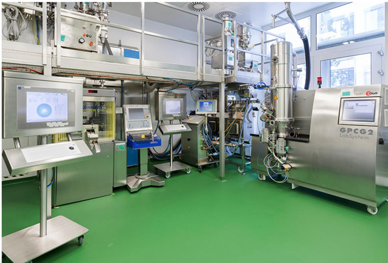
Once the chemical reactions are complete, pill production begins. The system dries and granulates the active substance and compresses it into tablets. Image by Tanja Devald/Novartis.
