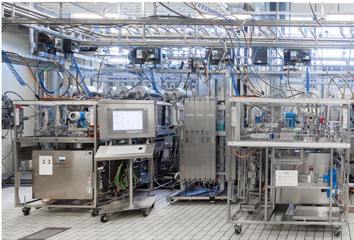
With continuous manufacturing, chemicals flow through multiple vertical chemical reactors that perform sequential reactions. Computer software controls the reactions and assesses quality. Image by Tanja Devald/Novartis.
