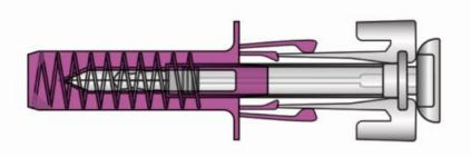
After the medicine has been injected the syringe guard will be activated to cover the needle. This is intended to protect against accidental needle stick injuries.
